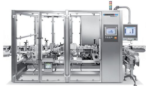
CPS 0600 integration kit, here integrated into 3rd party bottle labeling machine including helper code application on the bottom/cap
