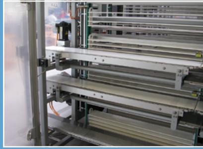
1 Row duplication: For an efficient and low-cost utilization of the buffering capacity. 2 Double output: Simple cleaning through retractable cross feeding conveyor. 3 Gondolas: Chocolate bars on coated shelves
