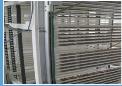
1 Row duplication: For an efficient and low-cost utilization of the buffering capacity. 2 Double output: Simple cleaning through retractable cross feeding conveyor. 3 Gondolas: Chocolate bars on coated shelves
